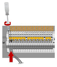
You can also connect the root and the normally open contact (see also Chapter **5.2 ALTERNATIVE OPERATING** mode).
