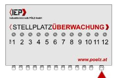
6. Push the connecting cable of the potential-free relay/alarm through the respective cable bushings on the front
